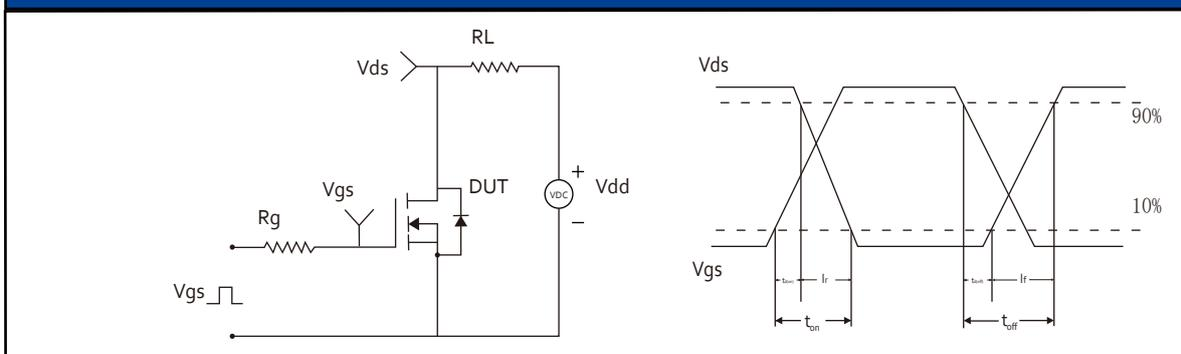
Fig.19 Unclamped Inductive Switching (UIS) Test Circuit & Waveforms
